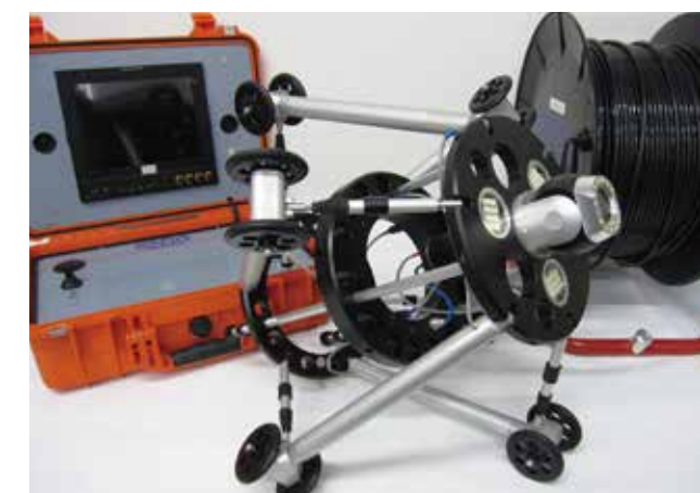
A Piping Inspection Robot for Large Diameter Pipes
